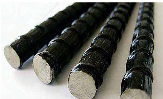
**Fig. 1.** Carbon fiber-reinforced polymer (CFRP) rods
